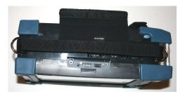
**8.** Fold the large part of the handle over the straps, and secure it in place with the Velcro.
