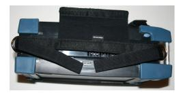
**7.** Fold the Velcro straps towards the center. Both ends should meet without any gap.
