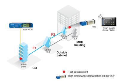
Figure 3. Link certification in a PON architecture with end-to-end connectivity.
