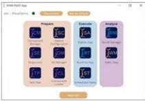
Full software suite for automation and control of test station, instruments and data. Allows users to define and maintain a logical structure among circuit components, design parameters, simulation results, experimental results and conditions, computations results and sequences. This provides all support needed for absolute traceability and reliability while naturally creating a dataset that is report-ready and AI-ready. |
