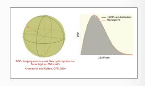
**Consequences of PMD compensation failures** - Bursts of error increasing the bit error rate (BER) - Loss of tracking and long recovery time, sometimes up to 20 seconds
