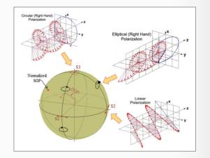
SOP changes randomly in real fibers - SOP rate of change follows a Rayleigh probability distribution.
