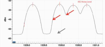
Case 2: ROADM present in the network - A ROADM contains filters that reduce interchannel noise - The traditional interpolation method leads to an underestimation of the noise - This creates a false sense of security
