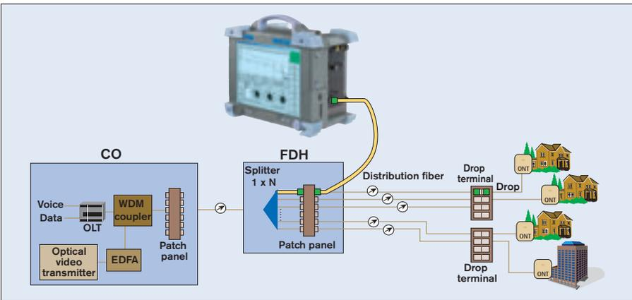
Figure 5.13 -- OTDR test between the FDH and CO
