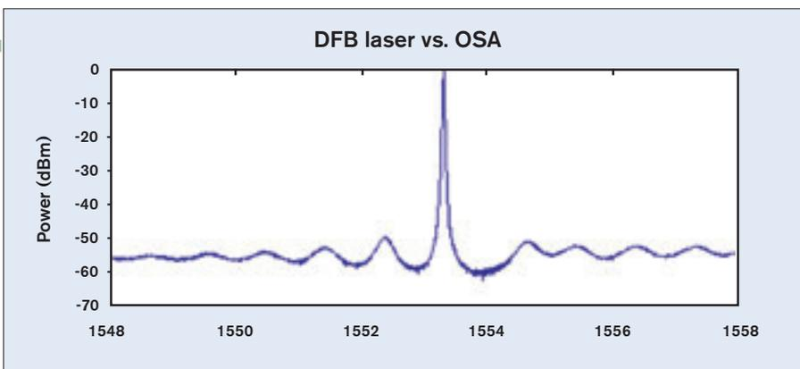
Figure 5.34 – Example of DFB laser spectral power distribution with an OSA
