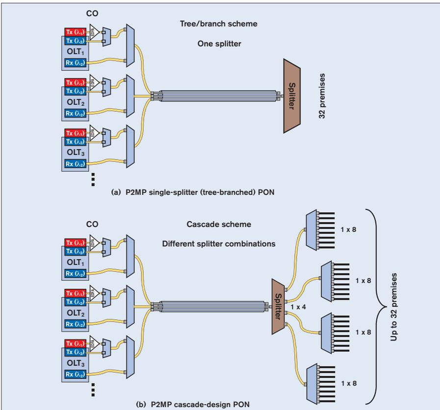
Figure 1.9 – Examples of point-to-multipoint (P2MP) networks
