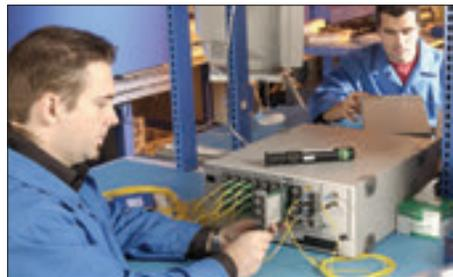
Figure 5.27 –PON passive component testing during manufacturing
