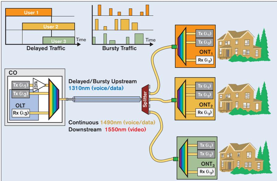
Figure 3.32 – Downstream and upstream traffic types
