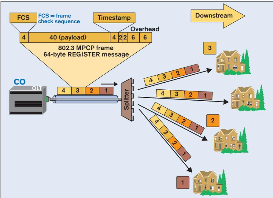
Figure 3.69 -- Downstream GATE register message process
