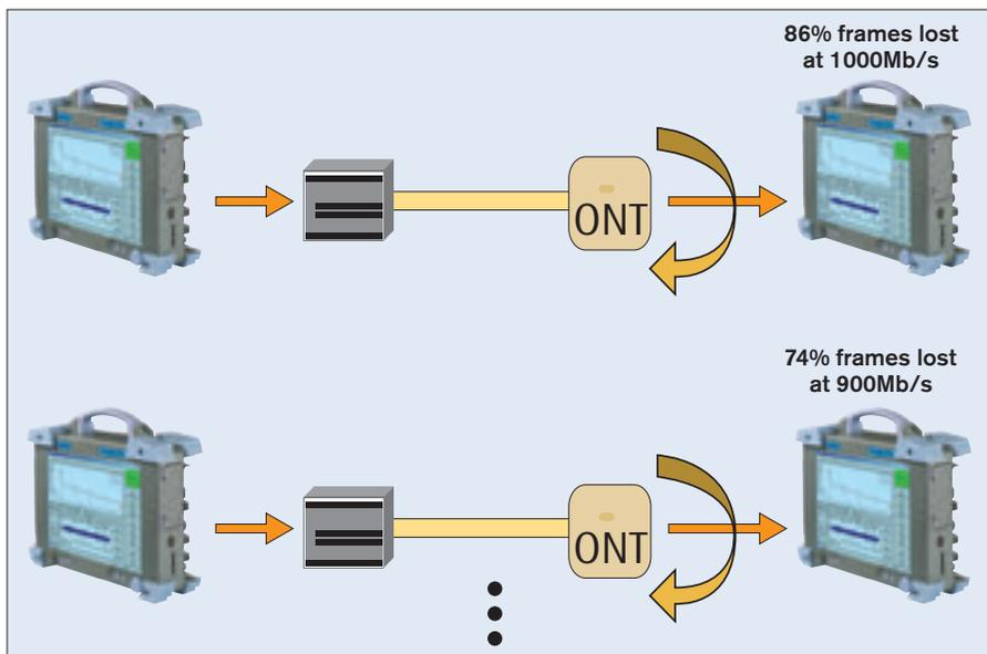
Figure 5.23 – Frame loss test
