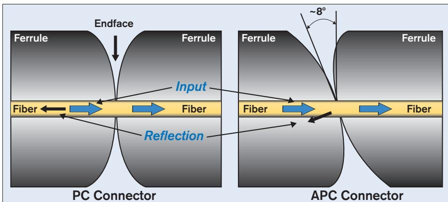
Figure 4.2 – Comparison between PC and APC connectors
