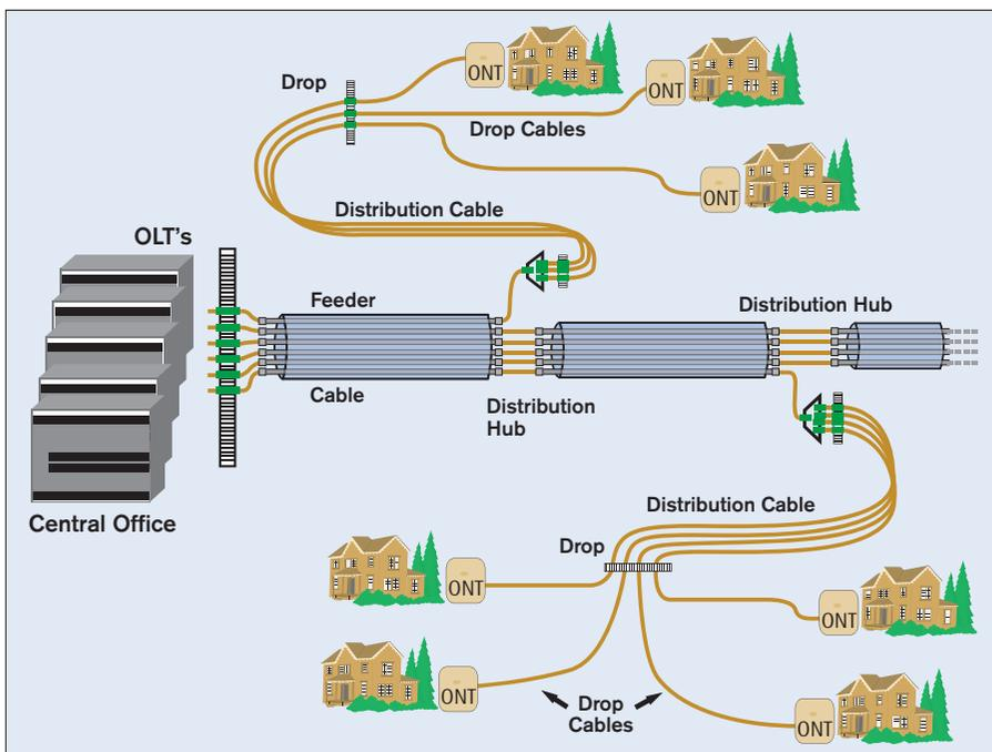
Figure 3.58 – Passive P2MP EPON topology using single fibers and splitters
