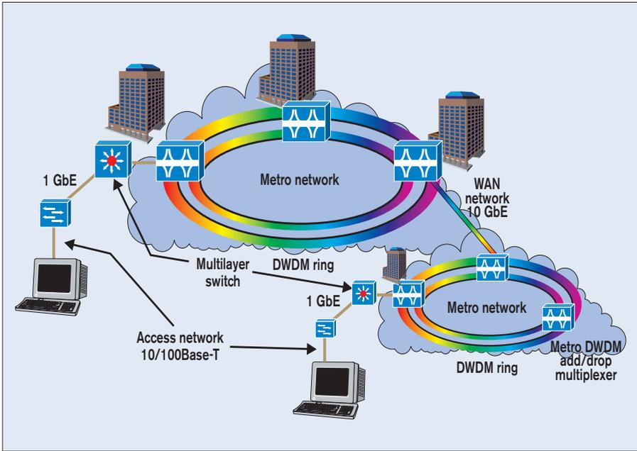
Figure 3.54 -- Ethernet in access networks, MAN and WAN
