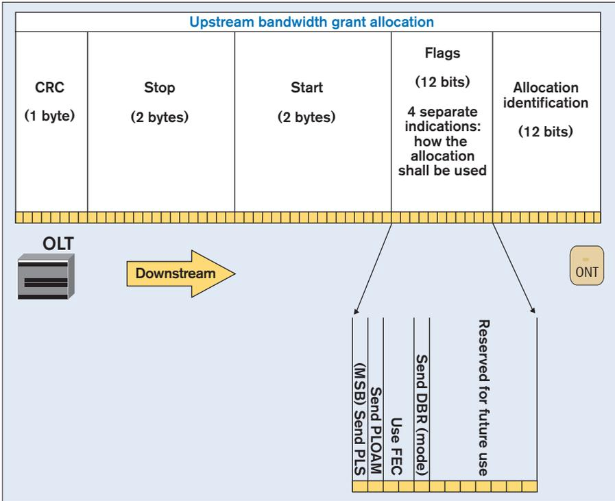
Figure 3.44 – Indication flags in the upstream bandwidth grant allocation block
