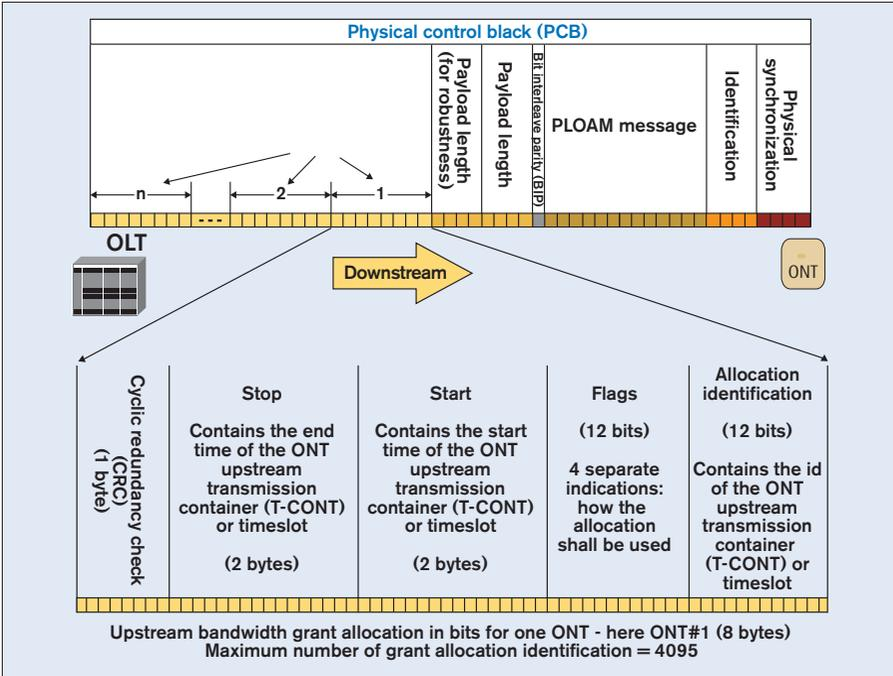
Figure 3.42 – Upstream bandwidth grant allocation block in the downstream physical control block
