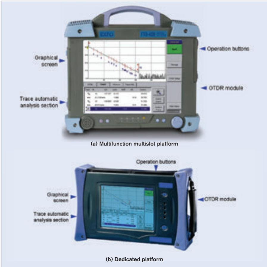
Figure 5.7 – Typical OTDR for field measurements
