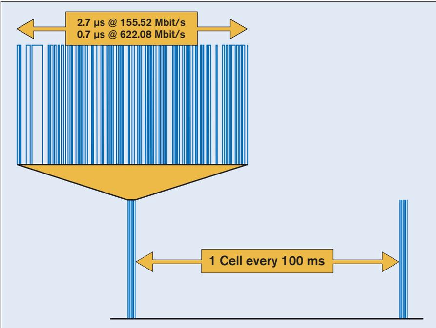
Figure 5.17 – Transmission of one BPON cell every 100 ms
