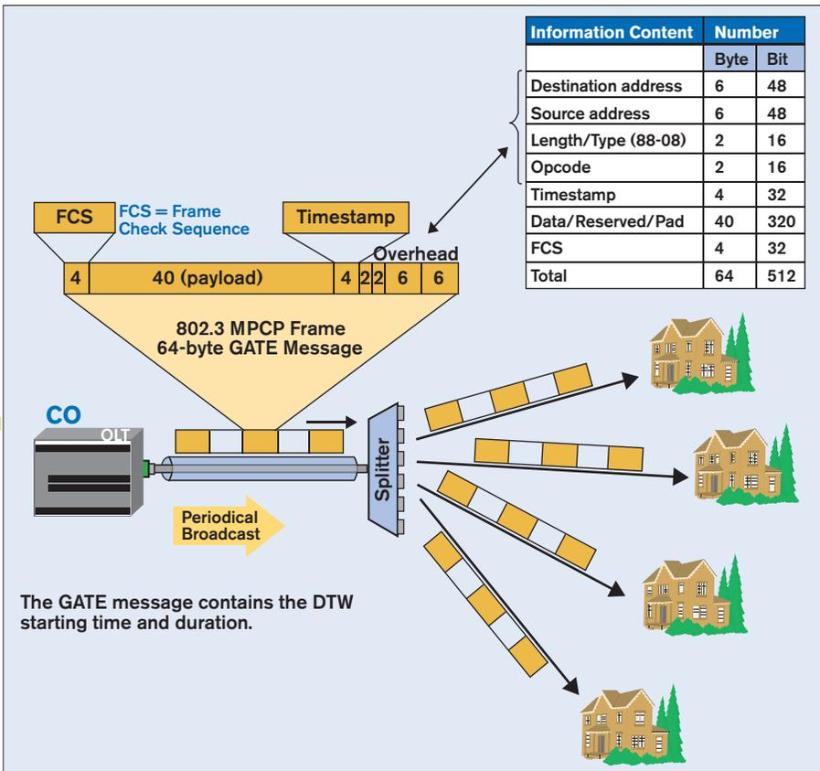
Figure 3.64 -- Downstream discovery process with GATE message
