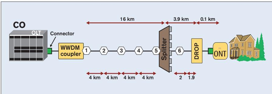
Figure 4.12 – Fiber length and splice scenario for a particular PON deployment
