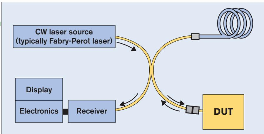
Figure 5.5 – Design schematic of an ORL test meter
