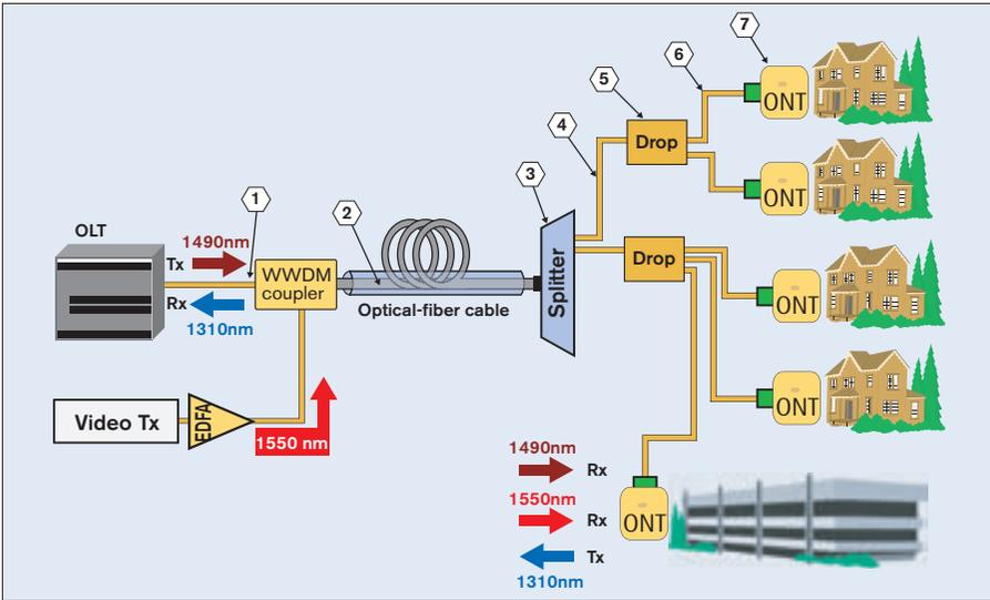
Figure 5.18 – Example of potential problem-causing locations in a complex PON topology
