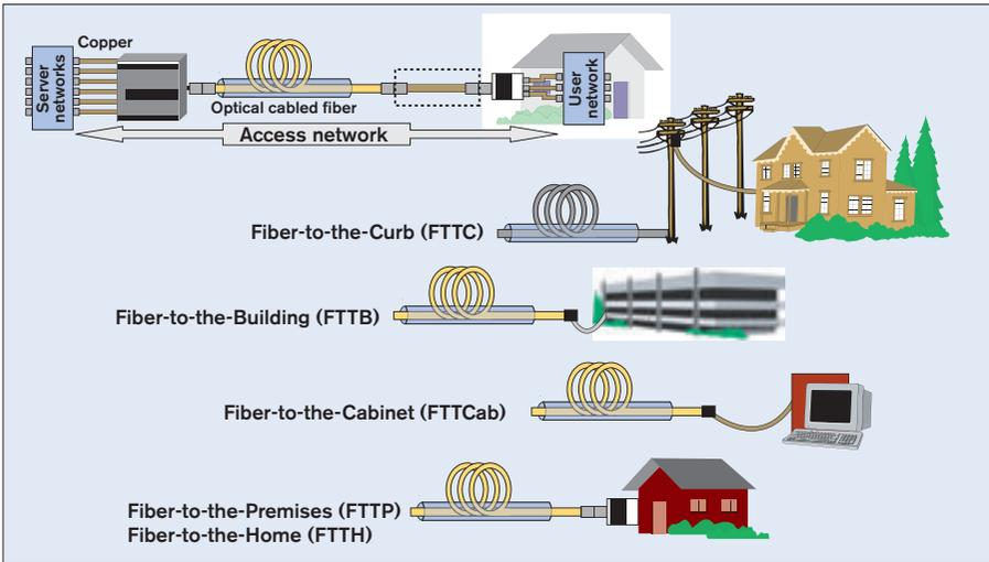
Figure 1.8 – Variations of the access network architecture
