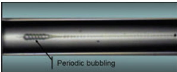
Figure 3.29 – Periodic bubbling in fiber core due to fusion splicing
