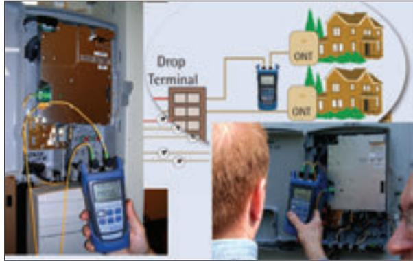
Figure 5.15 – PON ONT pass-through traffic test with a PON-optimized power meter
