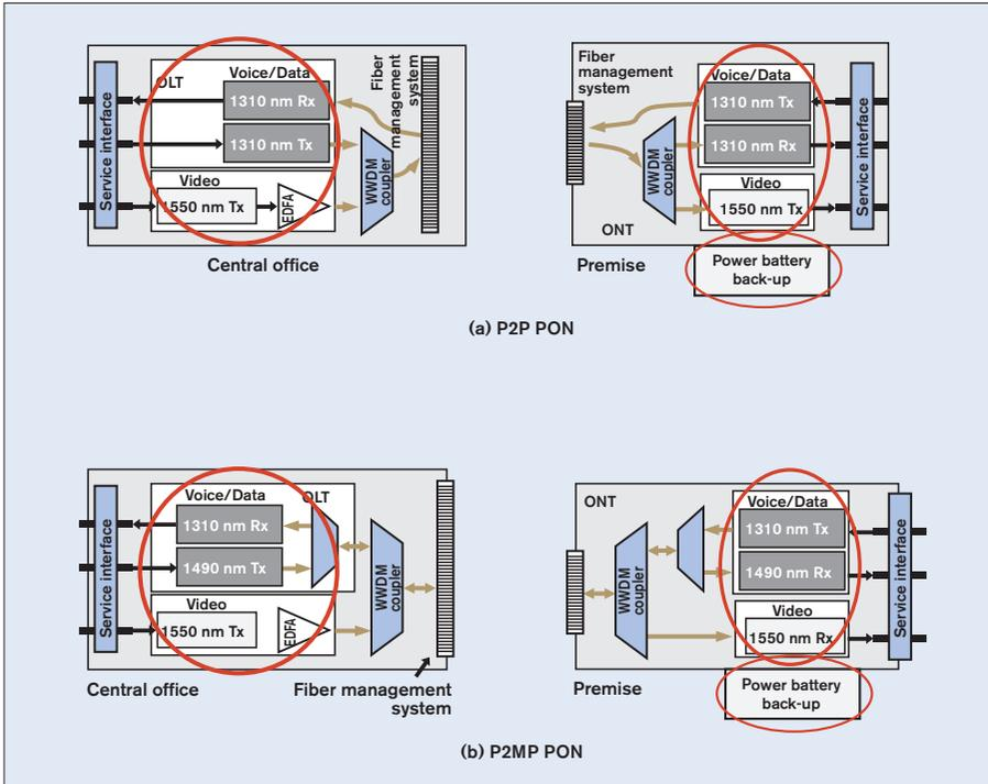
Figure 3.3 – PON active equipment for both P2P (a) and P2MP (b)
