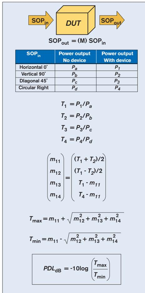
Figure 5.32 – PDL test procedure based on Mueller matrix
