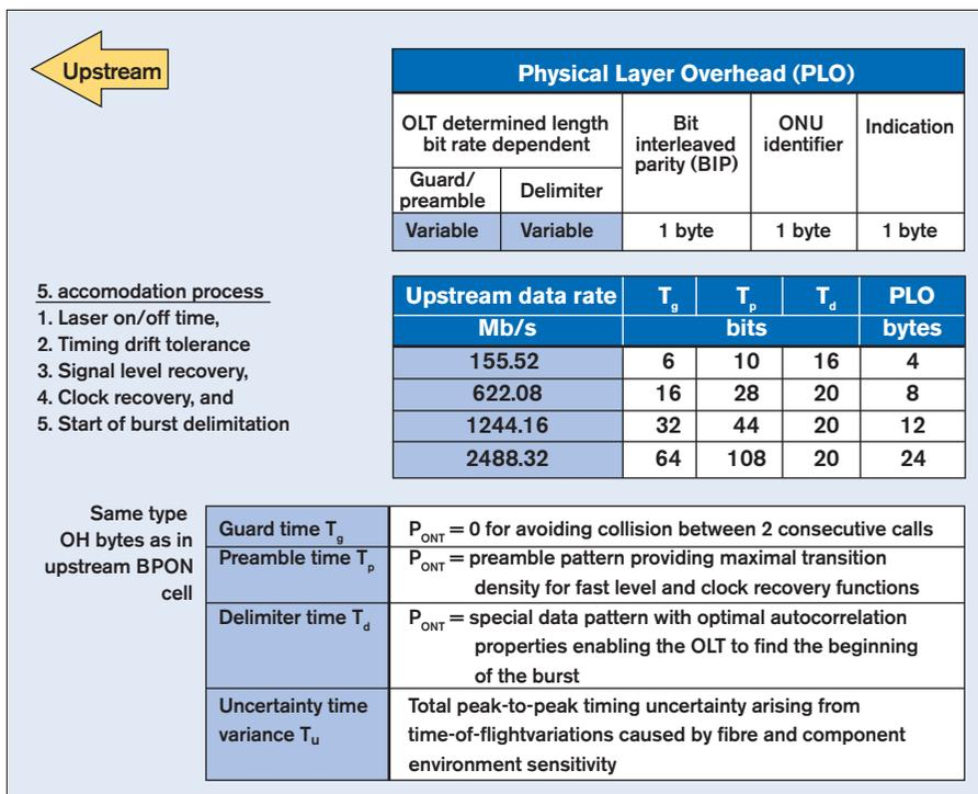
Figure 3.48 – Detailed byte and process structures of the upstream physical-layer overhead
