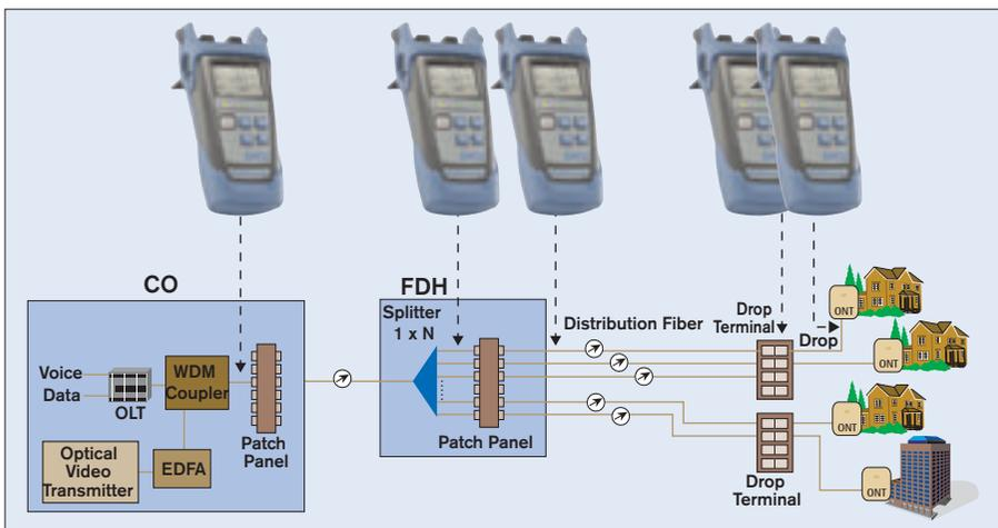
Figure 5.19 – Using a PON wavelength-isolating power meter for troubleshooting
