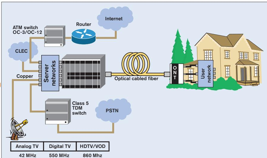
Figure 2.1 – FTTH PON basic system architecture
