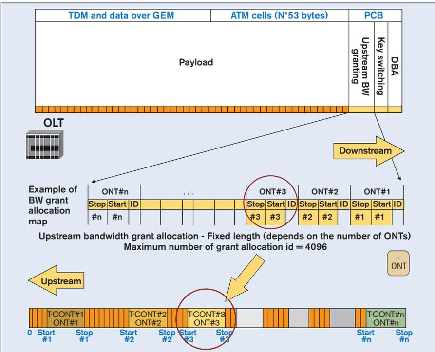
Figure 3.43 – Management of the upstream T-CONT transmission from the downstream physical control block
