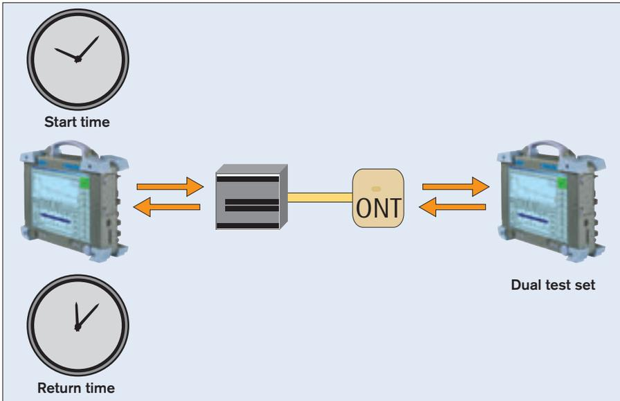
Figure 5.24 – Round-trip latency test
