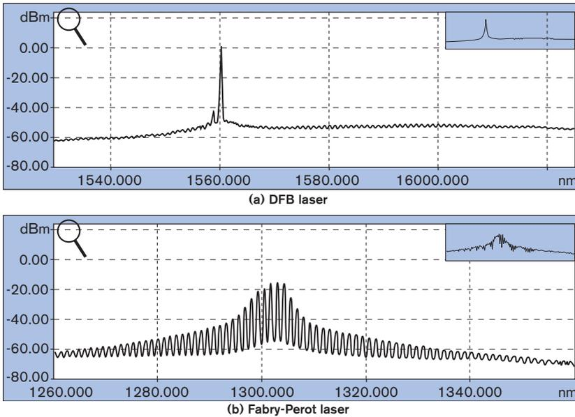
Figure 3.6 – Examples of wavelength spectra of the lasers used in FTTH PONs
