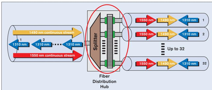
Figure 3.11 – Bidirectional 1 x N PON splitter
