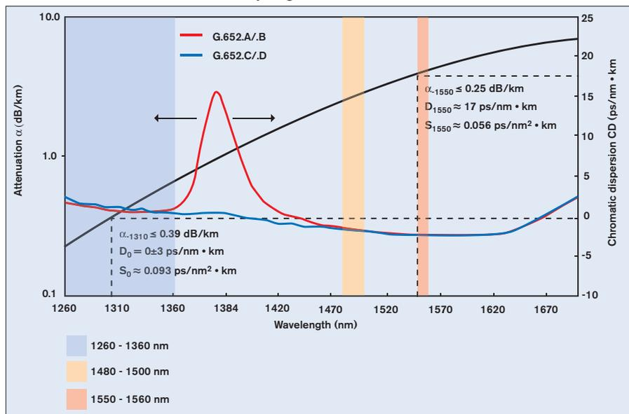
Figure 3.20 – Typical chromatic dispersion and spectral attenuation of FTTH PON fiber
