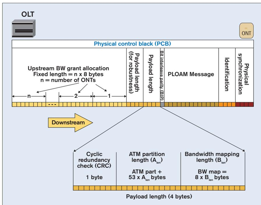
Figure 3.46 – Payload length block in PCB header
