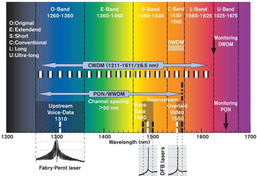
Figure 2.5 – FTTH P2MP PON wavelength allocation
