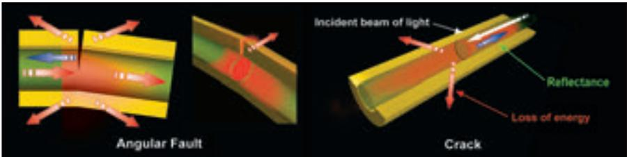
Figure 3.27 – Angular fault and crack when connecting two fibers
