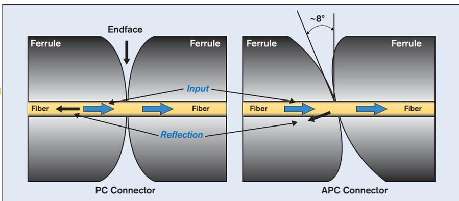
Figure 3 15 – Difference between PC and APC connectors
