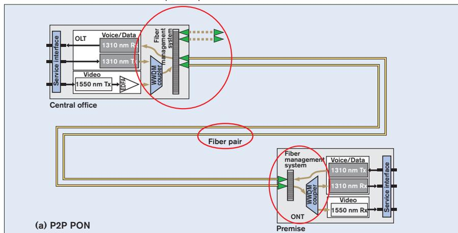
Figure 3.8a – PON passive components
