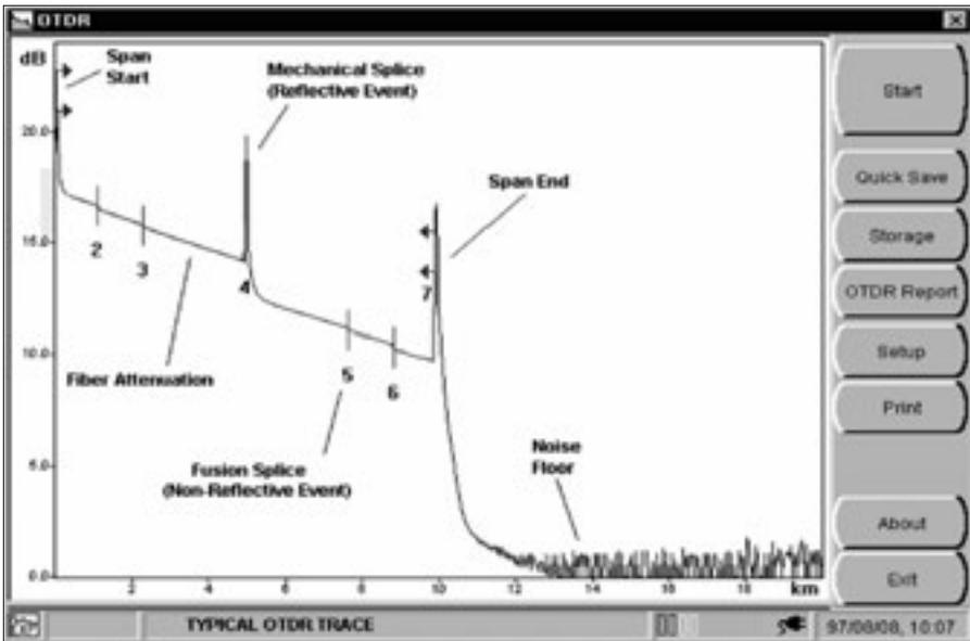
Figure 5.11 -- Example of OTDR test results
