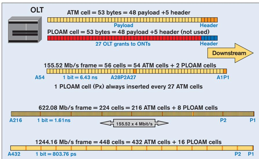
Figure 3.35 – BPON downstream ATM frame with PLOAM insertion
