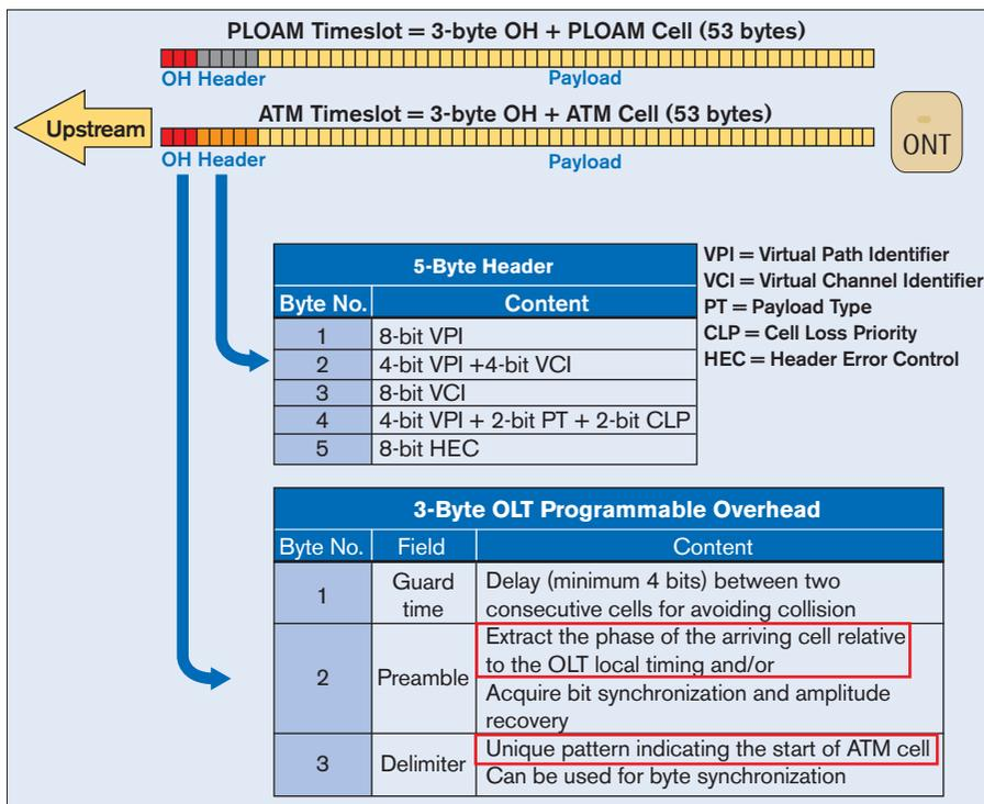
Figure 3.38 – Detailed timeslot byte structure
