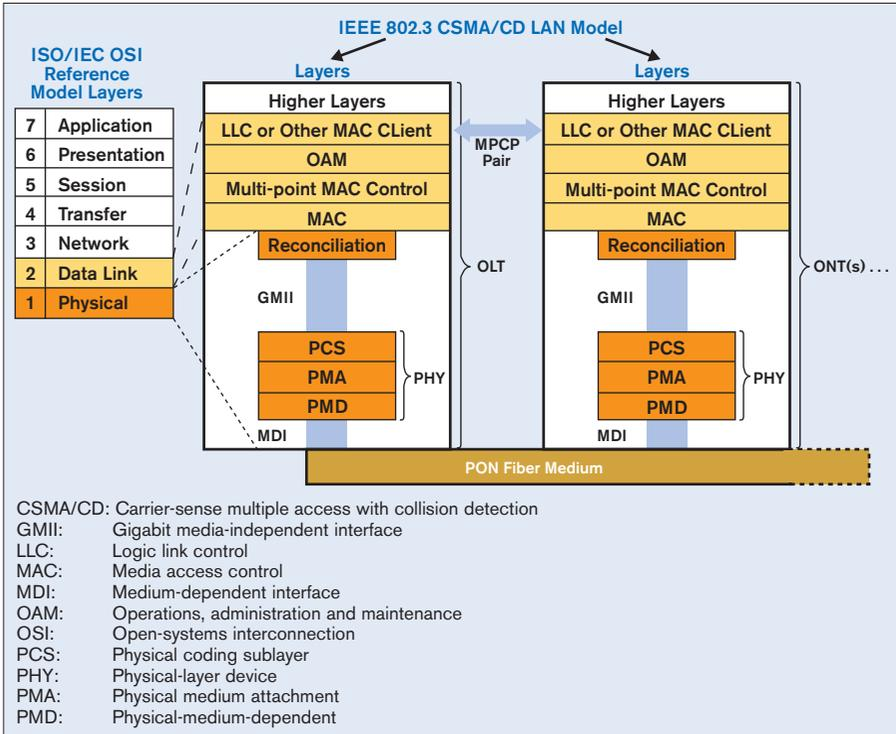
Figure 3.61 – EPON P2MP architecture
