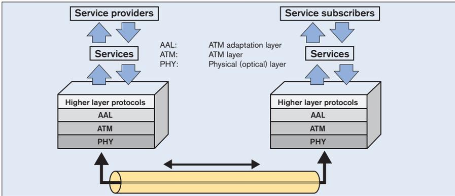
Figure 3.34 – Architecture ATM protocol service transmission structure
