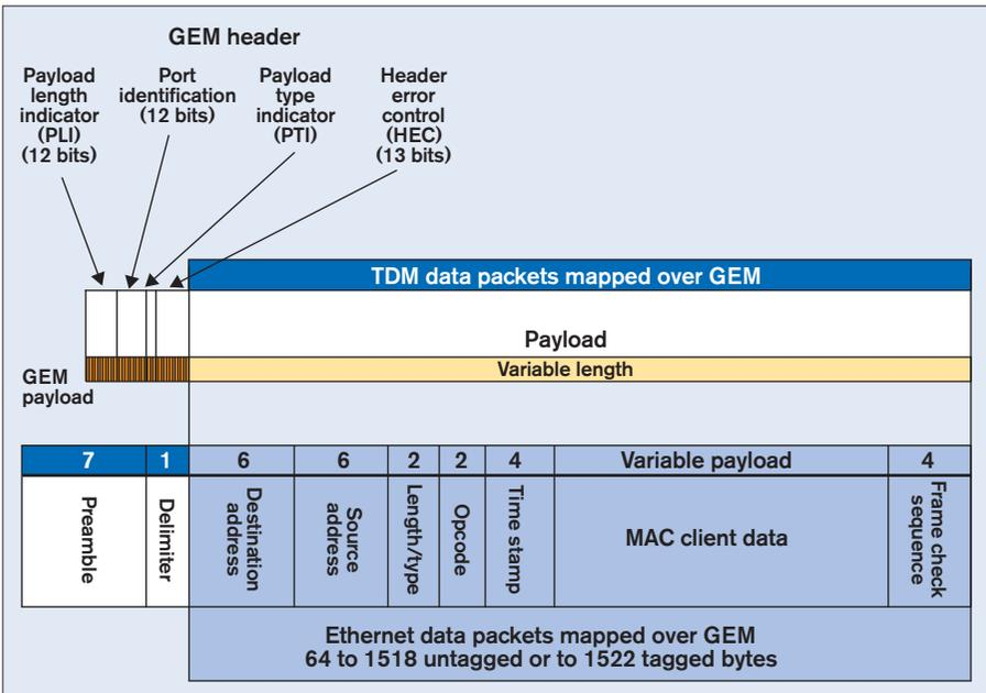
Figure 3.52 -- TDM and Ethernet transmission mapped over GEM
