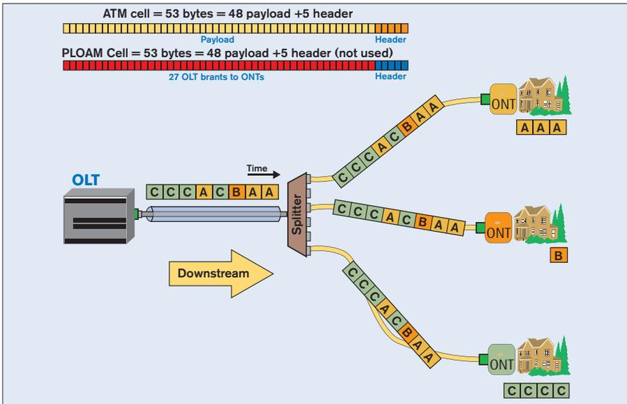
Figure 3.36 -- Downstream transmission
