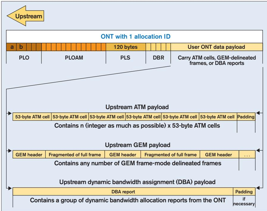
Figure 3.49 – GPON upstream payload types
