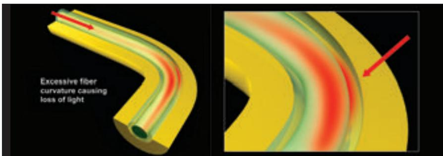
Figure 3.23 – Macrobending in optical fiber
