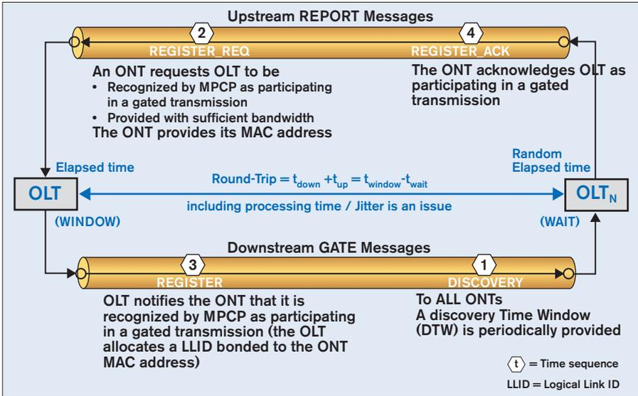
Figure 3.63 – Communication processing between the OLT and an ONT
