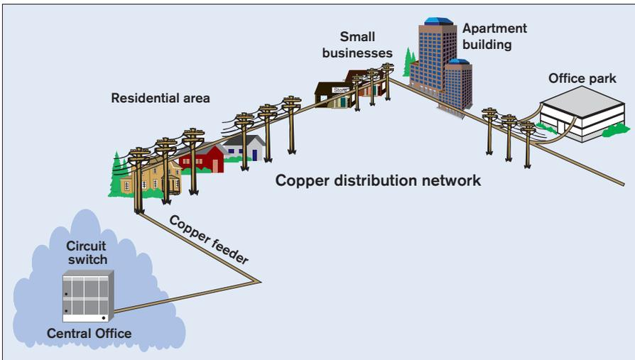
Figure 1.7 – Traditional copper-based access network
