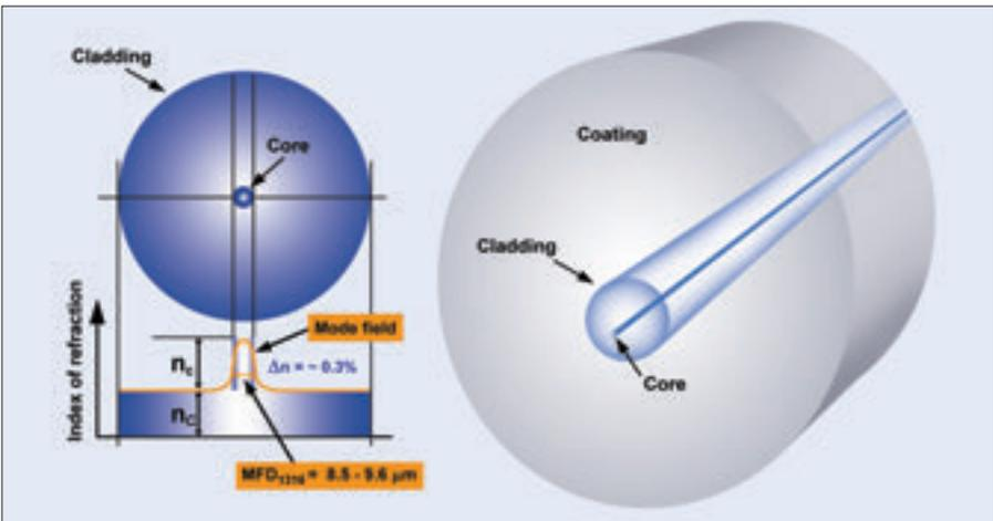
Figure 3.19 – Typical geometry of singlemode dispersion unshifted fiber used in PON
