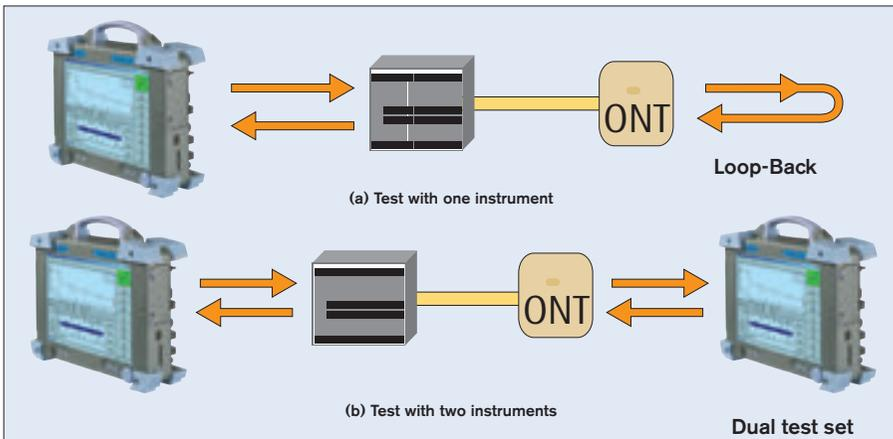
Figure 5.21 – Measuring throughput
