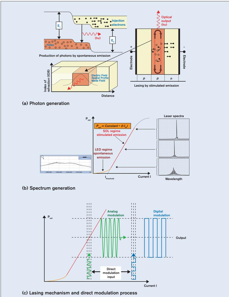
Figure 3.7 – Lasing mechanism in a semiconductor
