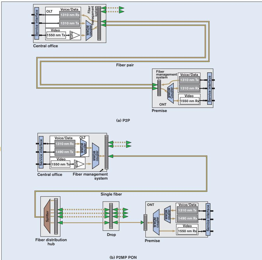
Figure 3.1 – Main PON components – basic system architecture [Pv1\_37]
