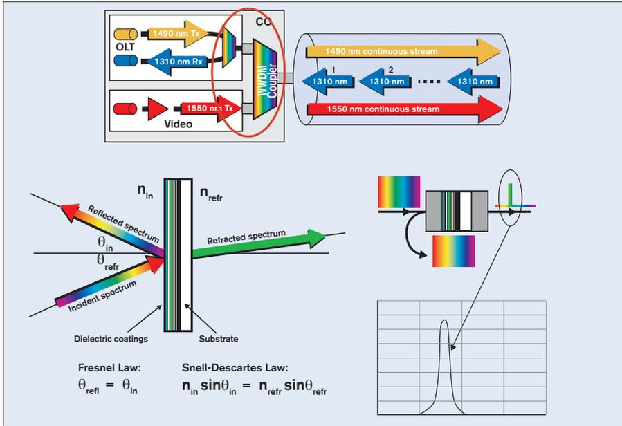
Figure 3.9 – Bidirectional Wide WDM (WWDM) three-port thin-film-filter coupler
