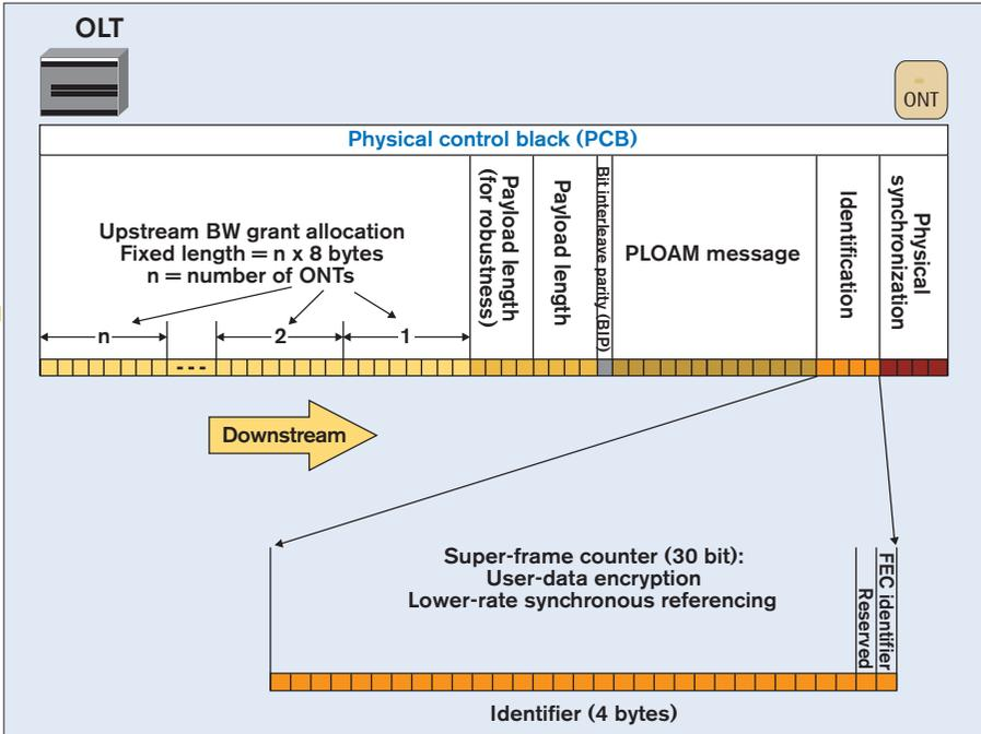
Figure 3.45 – Identification block in the PCB header
