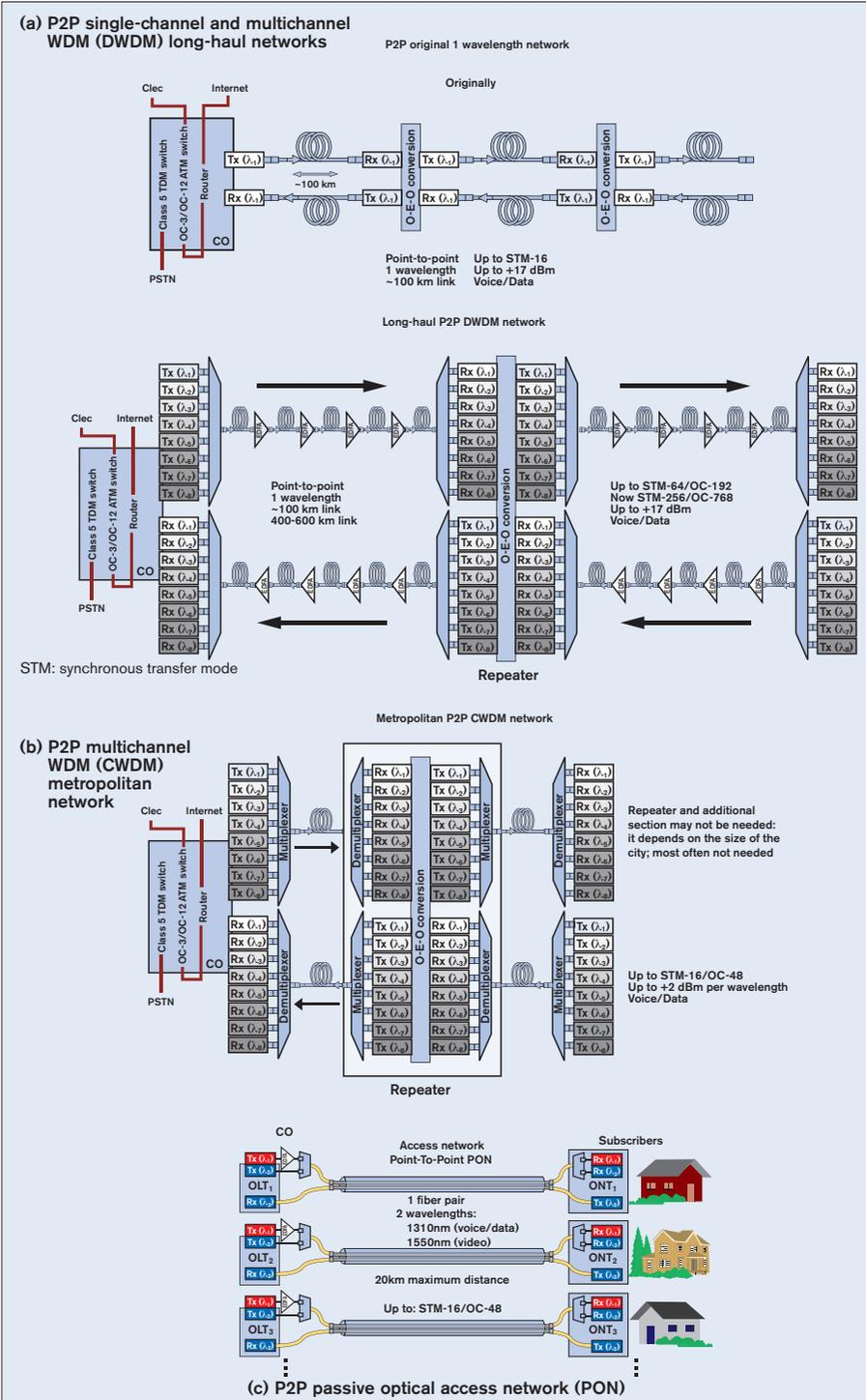
Figure 1.6 – Examples of point-to-point (P2P) optical networks
