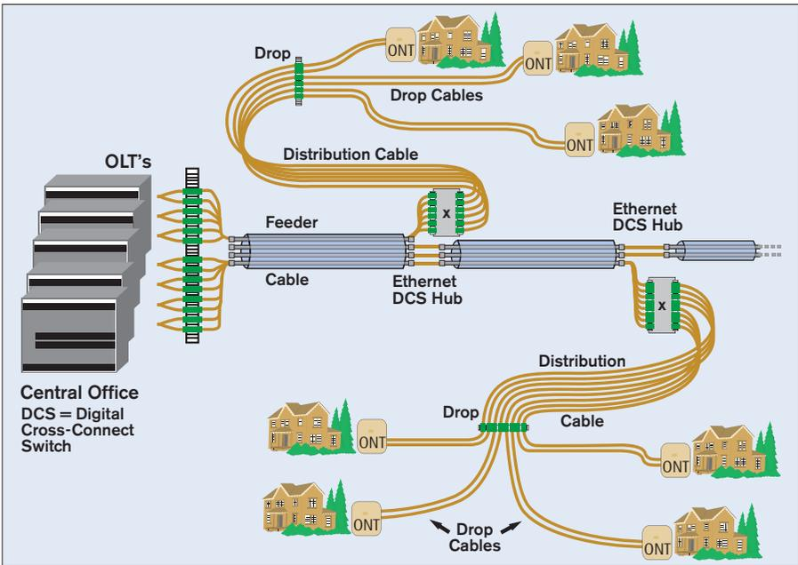
Figure 3.57 -- Active P2P Ethernet network topology using fiber pairs and switches (P2MP is also possible)
