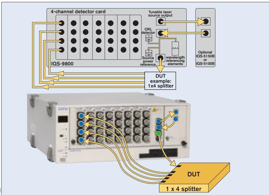
Figure 5.28 –PON test system for PON passive components
