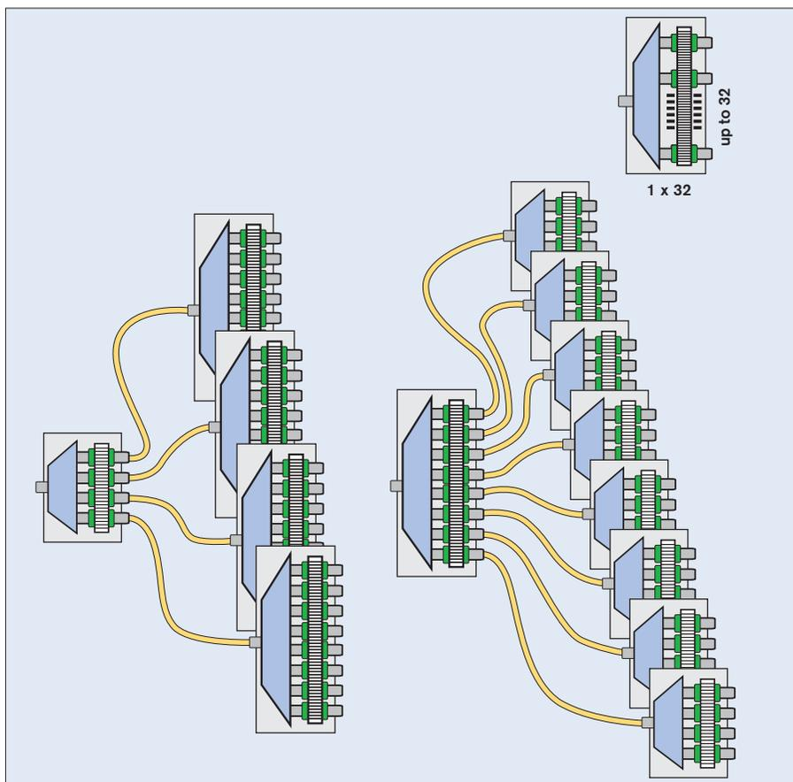
Figure 3.12 – Examples of various 1 x 32 PON splitter topology
