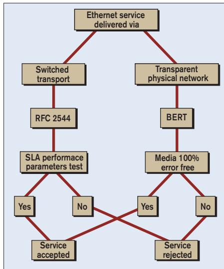
Figure 5.26 – Ethernet service acceptance testing functional diagram
