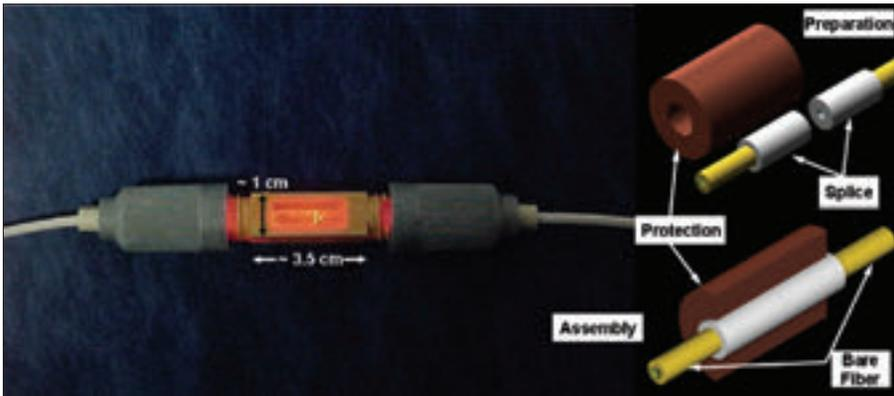
Figure 4.9 – Example of conventional mechanical splicing process
