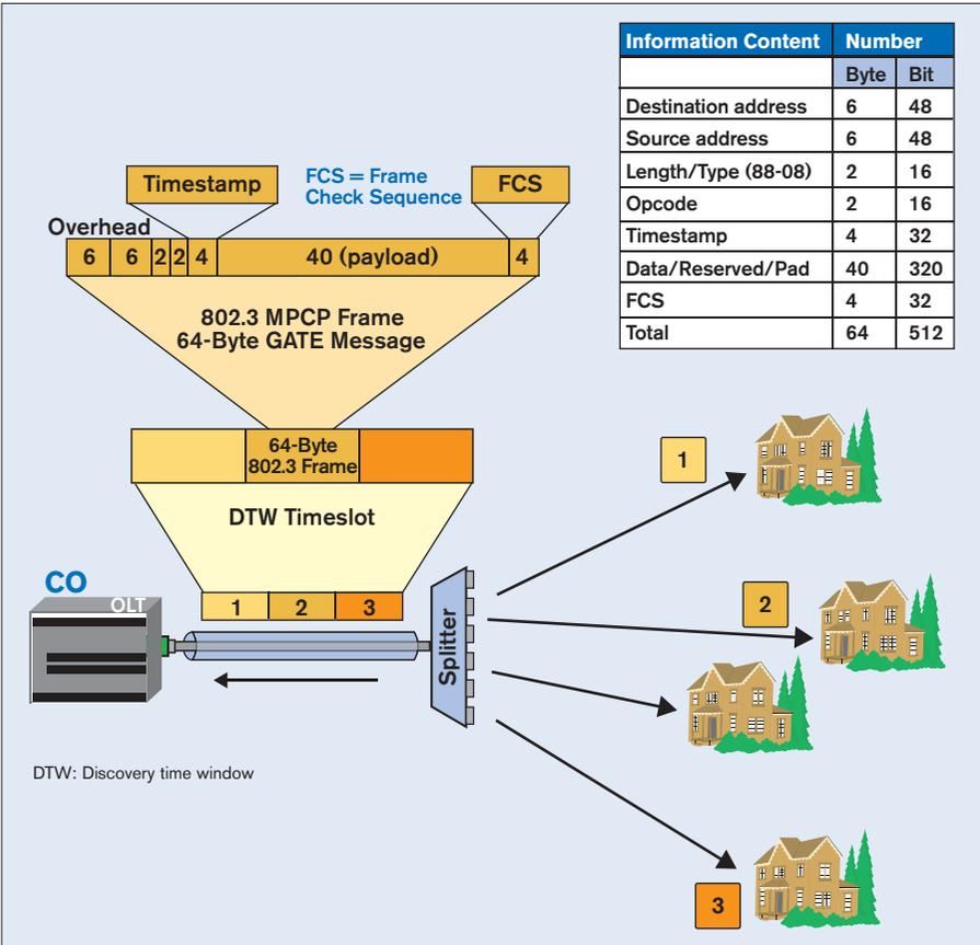
Figure 3.66 -- Upstream MPCP REGISTER\_REQ reporting process
