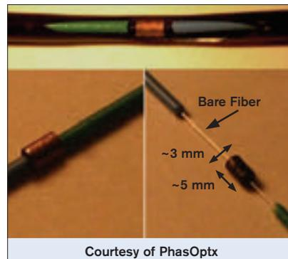
Figure 4.10 – Example of new mechanical splicing technology
