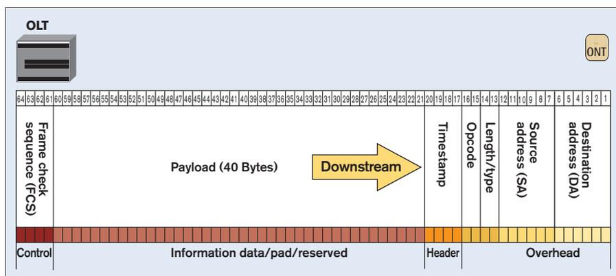
Figure 3.59 – Basic IEEE 802.3 frame structure
