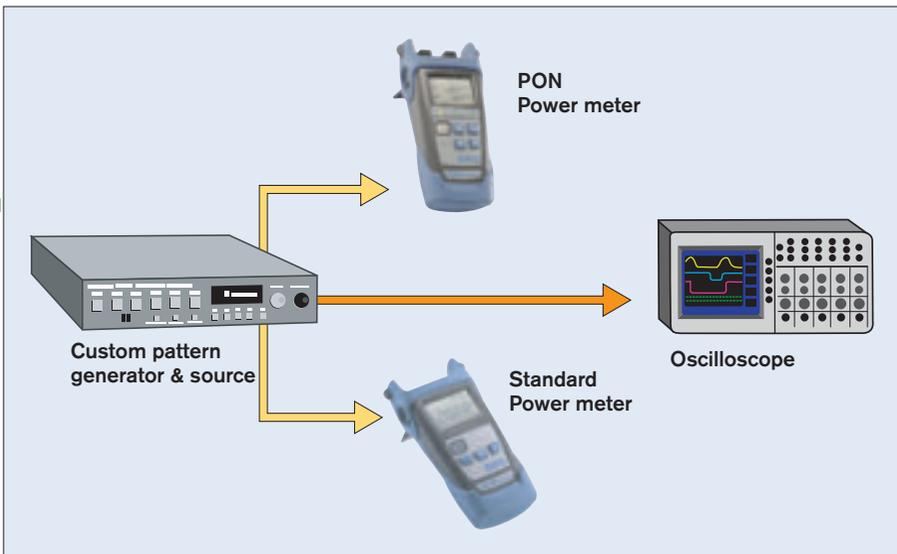
Figure 5.16 – Setup for performance comparison between a standard and a PON-optimized power meter in “bursty” traffic conditions
