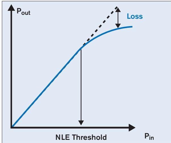
Figure 3.21 -- Power loss due to non-linear effects in a singlemode fiber
