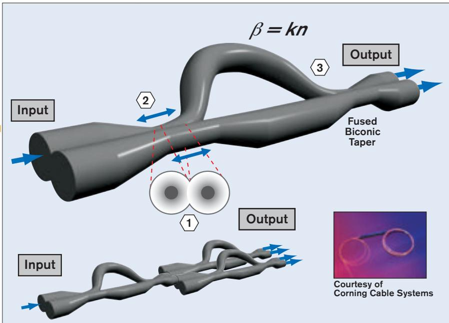
Figure 3.13 – Splitter design based on fused biconic tapered fiber (2 x N ratio is possible)
