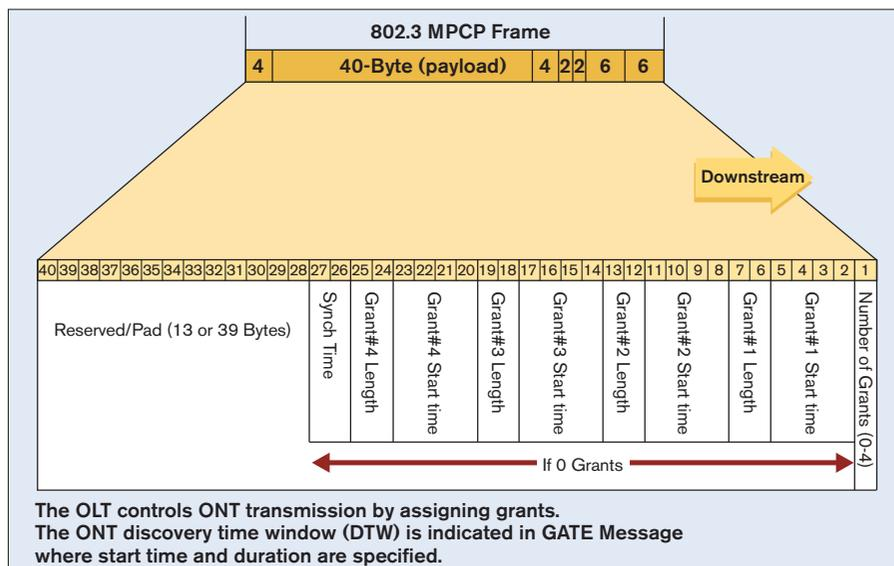
Figure 3.65 -- MPCP GATE granting message payload
