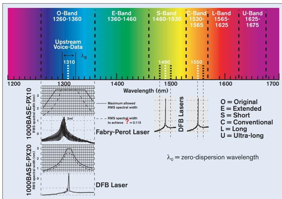
Figure 3.60 -- EPON wavelengths and bands
