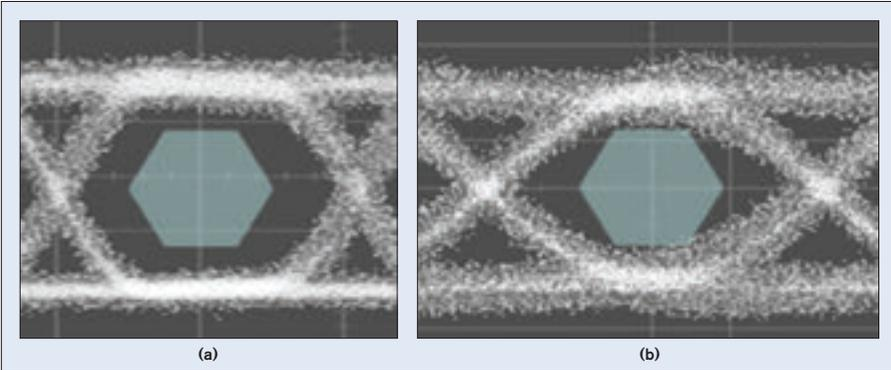
Figure 5.20 – Example of an eye pattern with hexagonal eye mask
