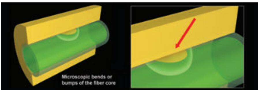
Figure 3.24 – Microbending in optical fiber
