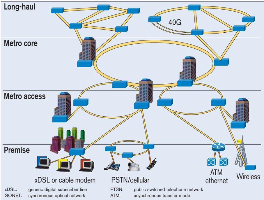
Figure 1.5 – Terrestrial fiber-optic networks
