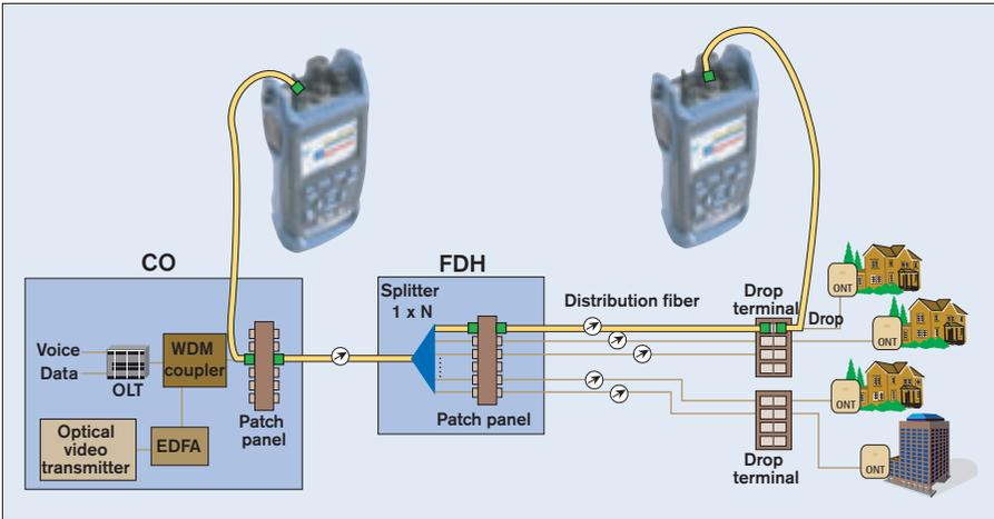
Figure 5.9 – Simultaneous optical loss and ORL measurements
