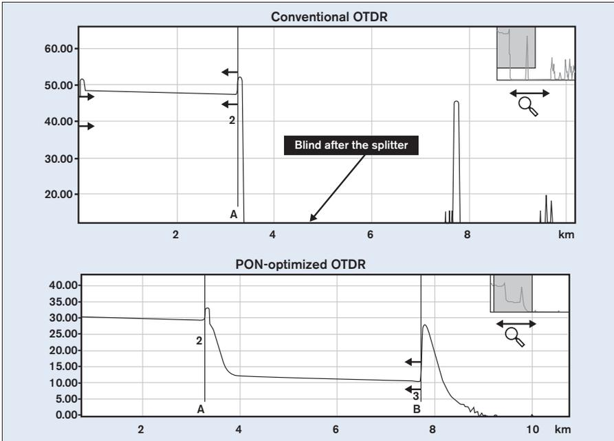
Figure 5.12 – Results from a conventional and a PON-optimized OTDR [P147 from “Testing and Maintaining FTTH PONs: New Challenges” - Stéphane Chabot]
