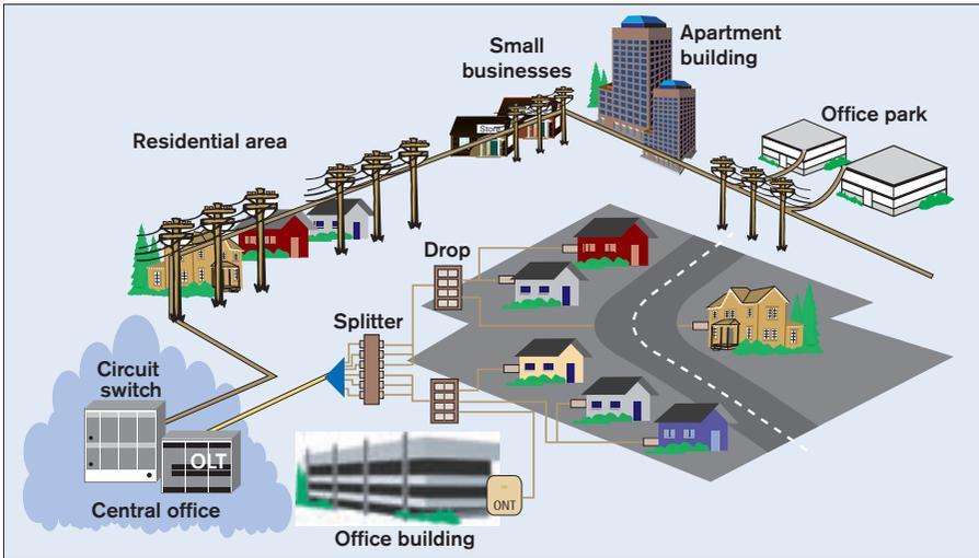
Figure 1.10 – Example of FTTH PON in new housing (Greenfield) development
