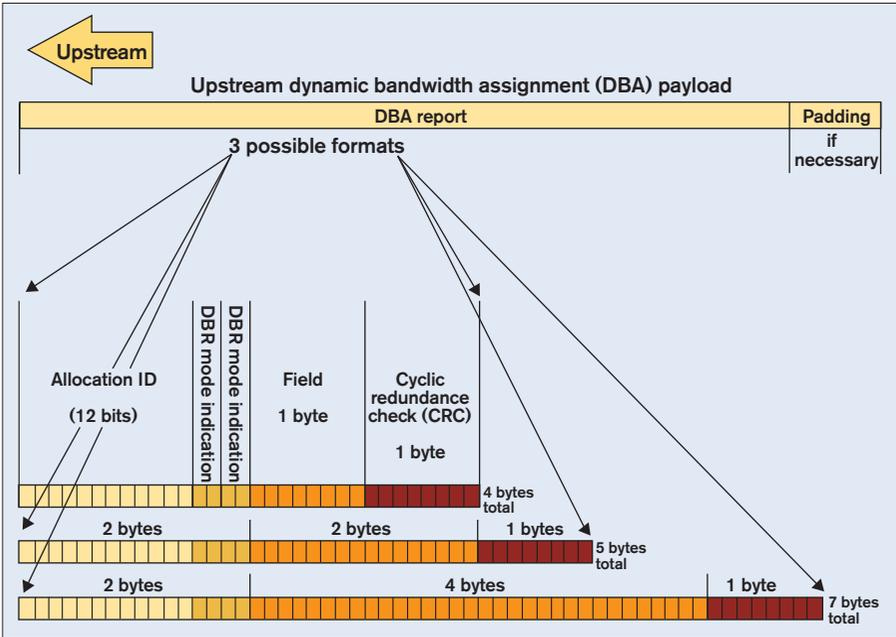
Figure 3.51 -- Upstream DBA payload
