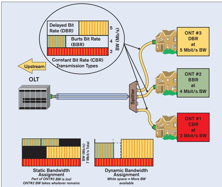
Figure 3.40 – Dynamic bandwidth assignment (DBA) compared to static bandwidth assignment (SBA)
