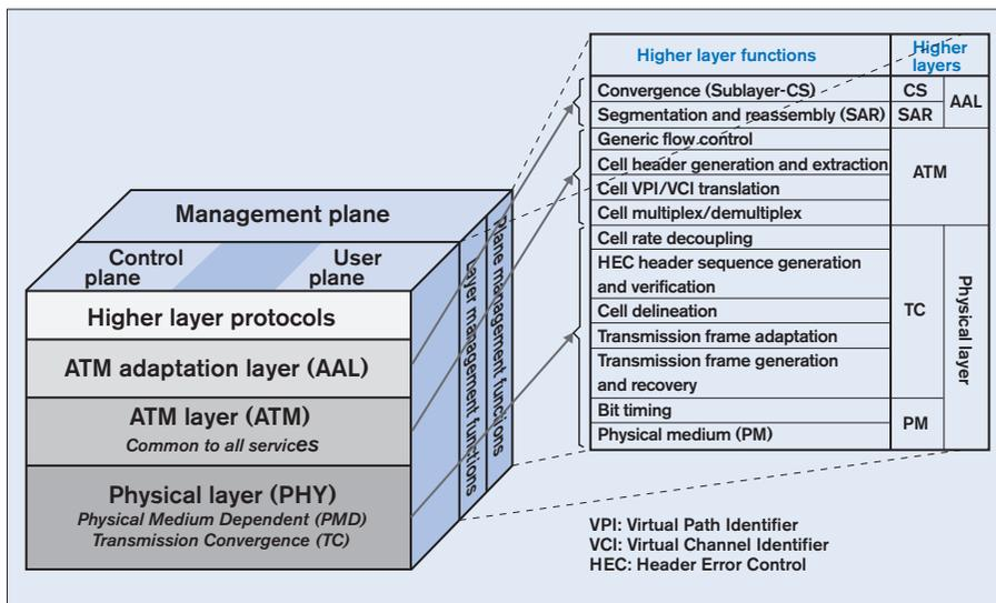
Figure 3.33 – The layer-based structure of the ATM protocol (ITU-T Rec. 1.371)
