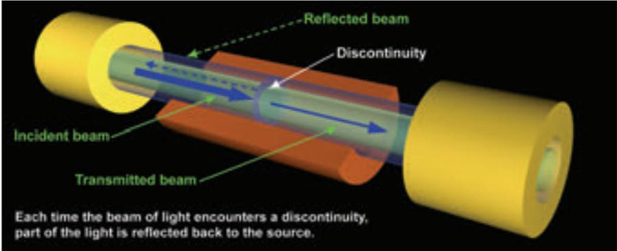
Figure 3.25 – Discontinuities, gaps or voids when connecting two fibers
