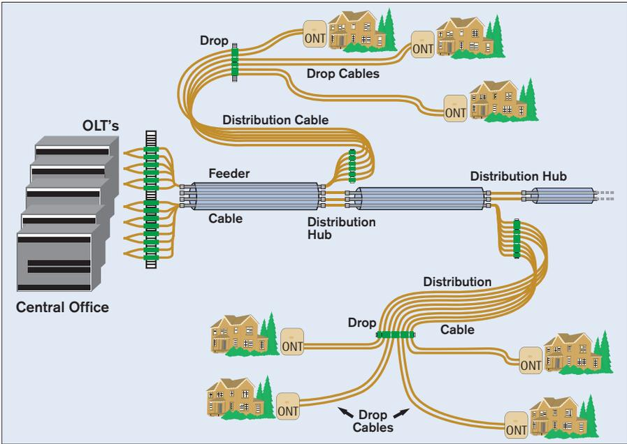
Figure 3.56 -- P2P Ethernet network topology using fiber pairs
