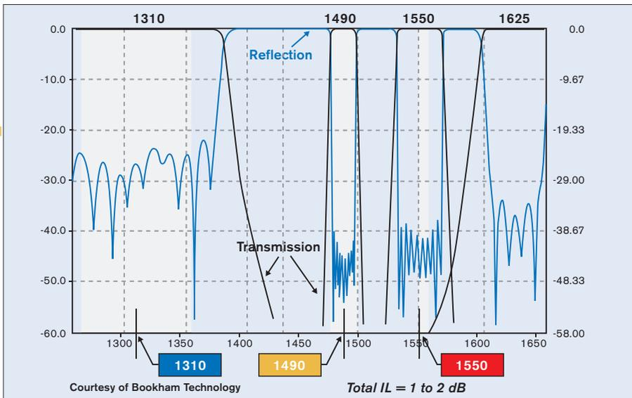
Figure 3.10 – Characteristics of typical PON WWDM coupler based on thin-film-filter technology
