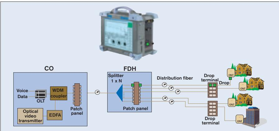
Figure 5.14 – OTDR test between the FDH and one ONT
