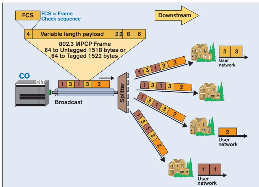
Figure 3.73 – EPON OLT downstream data broadcast transmission process
