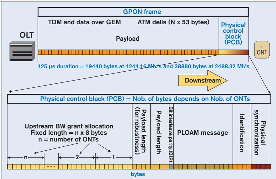
Figure 3.41 – GPON downstream frame and PCB header structure (BW=Bandwidth)
