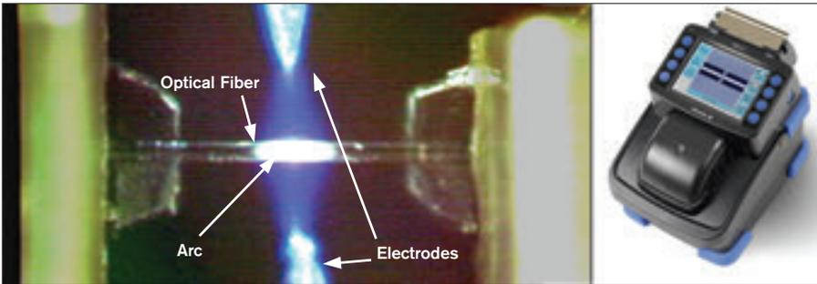
Figure 4.11 – Example of fusion splicing process and equipment
