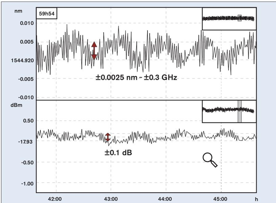
Figure 5.33 – Example of long-term optical source power and frequency stability
