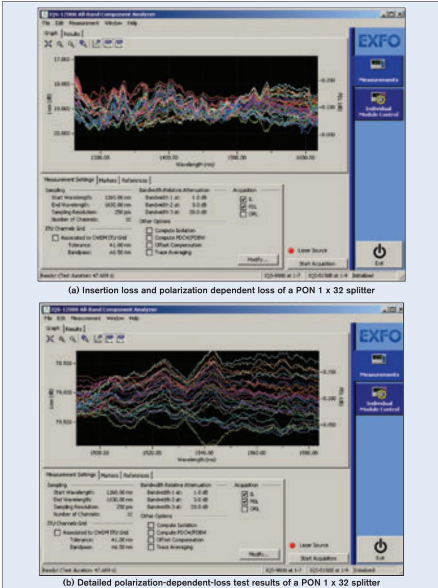
Figure 5.29 – Polarization-dependent-loss test results of a PON 1 x 32 splitter
