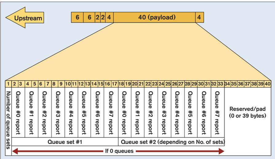
Figure 3.67 -- MPCP REGISTER\_REQ REPORT message payload
