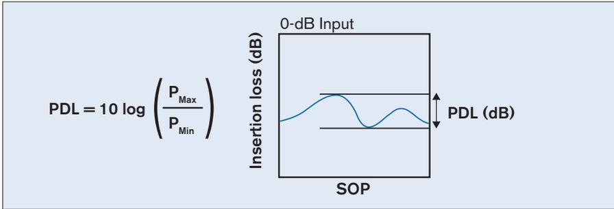
Figure 5.30 – Definition and measurement of polarization-dependent loss
