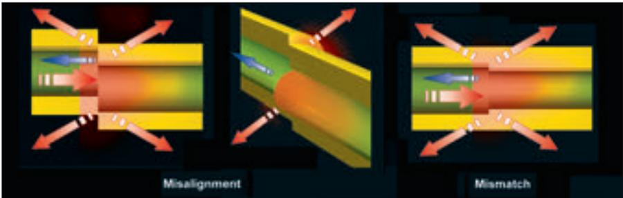
Figure 3.26 – Misalignments and mismatches occurring when connecting two fibers
