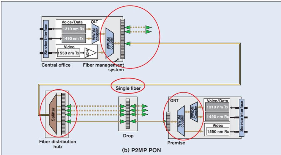
Figure 3.8b – PON passive components
