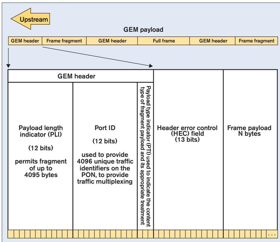
Figure 3.50 -- Upstream GEM payload header
