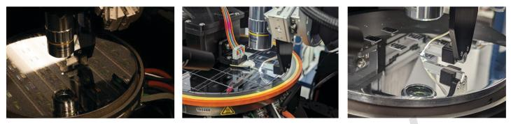
Figure 3. Re-testing the same circuits with a single OPAL-EC station over the process chain: from wafer, to singulated dies on stretch-tape, to multiple depopulated dies on a plate adapter. Here, with optical surface coupling and DC probe.
