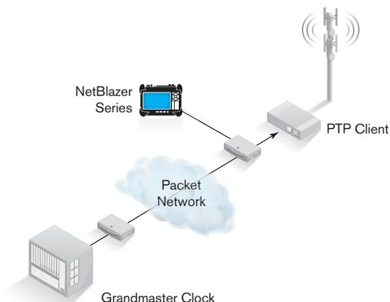
Figure 3. PTP testing using the NetBlazer
