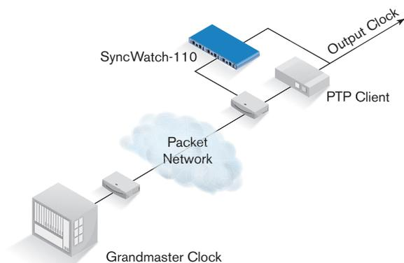
Figure 4. PTP performance testing with the SyncWatch-110
