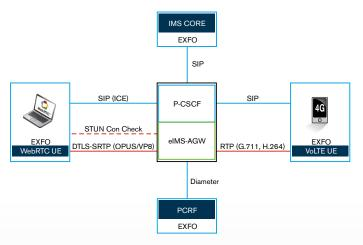
3) SBC supporting only the WebRTC media (eIMS-AGW) function together with a stand-alone WebRTC signaling gateway
