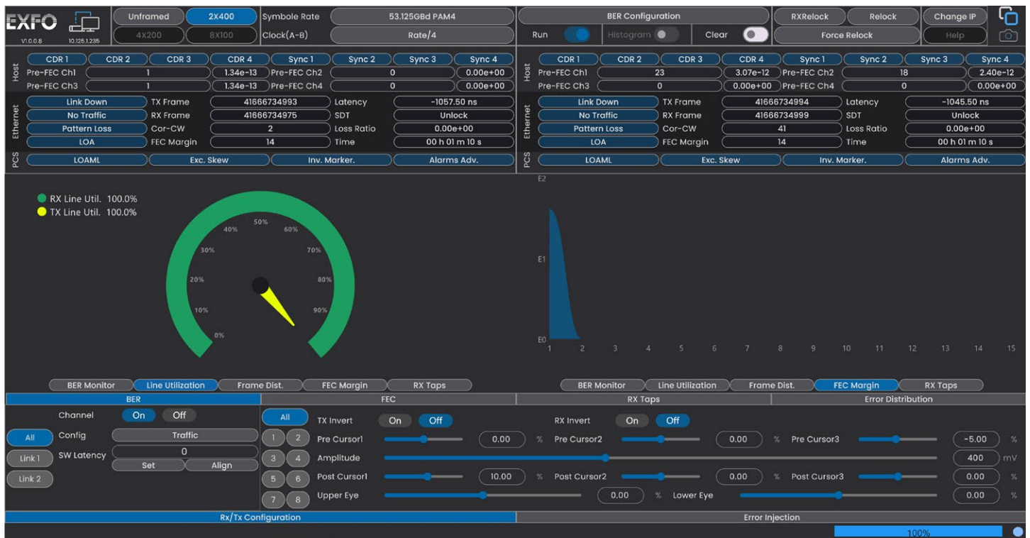
Figure 4. Test pre/post FEC BER, symbol error distribution and FEC margin.
