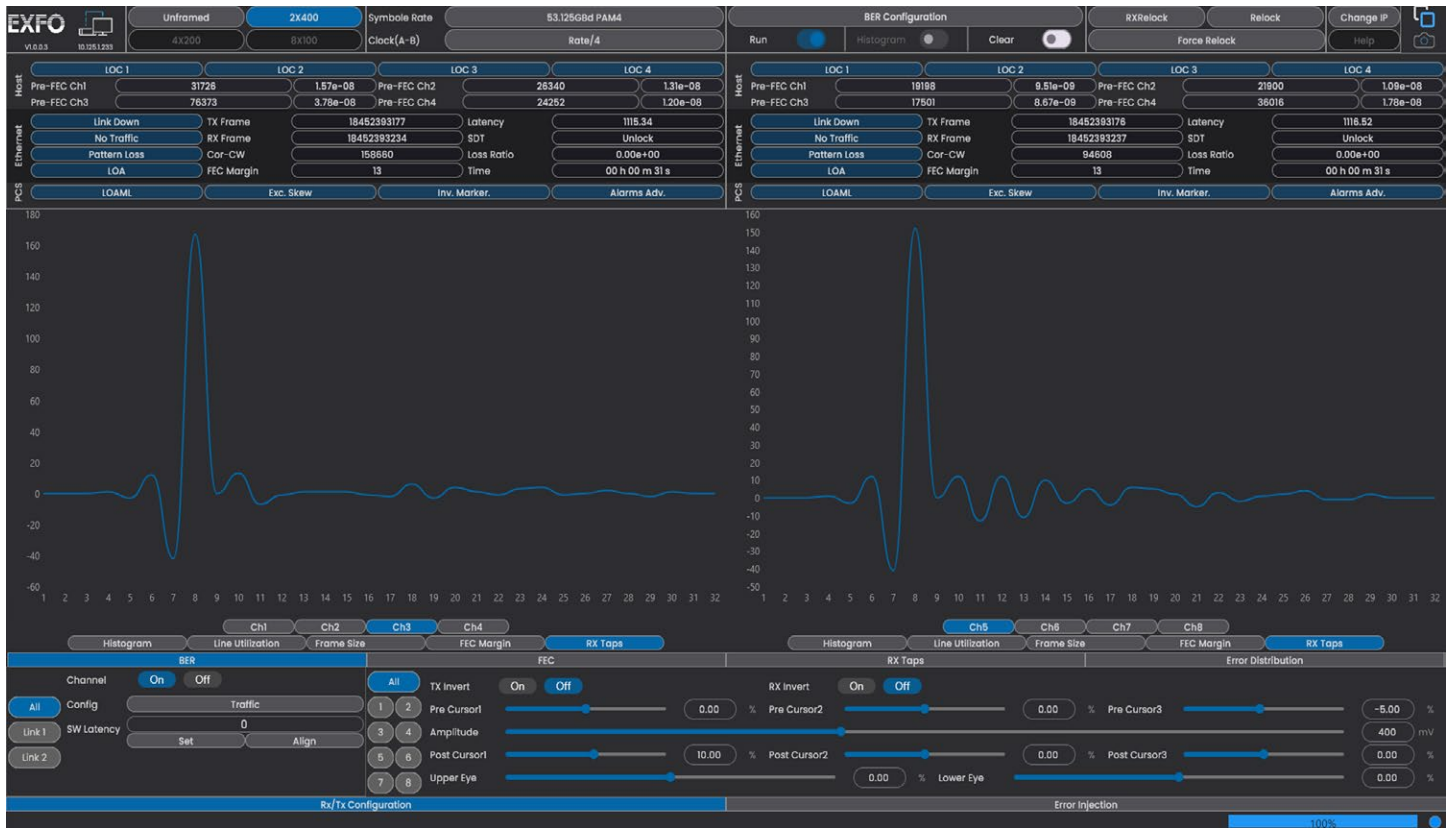
Figure 3. Detect ISI and far-end reflection.
