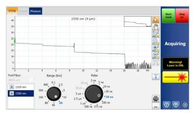
Dialing wheels allows to adjust real time acquisition parameters on the fly, immediately seeing the effect on the trace for optimal efficiency. Ready to launch the characterization? Just press the "start iOLM" button, no need to manually interrupt real time nor getting into any menus.
