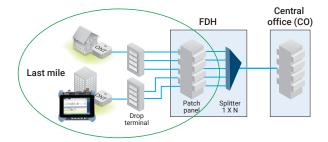
Figure 1. Certification of last-mile FTTH including continuity at splitter.
