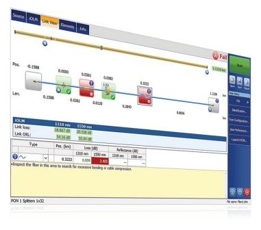
Simplify OTDR tests while optimizing characterization accuracy for all network topologies. iOLM is powered by intelligent algorithms that can adapt to the context. Still unmatched in the industry, iOLM dynamically locates and identifies all network components and faults with maximal resolution—all at the push of one button.
