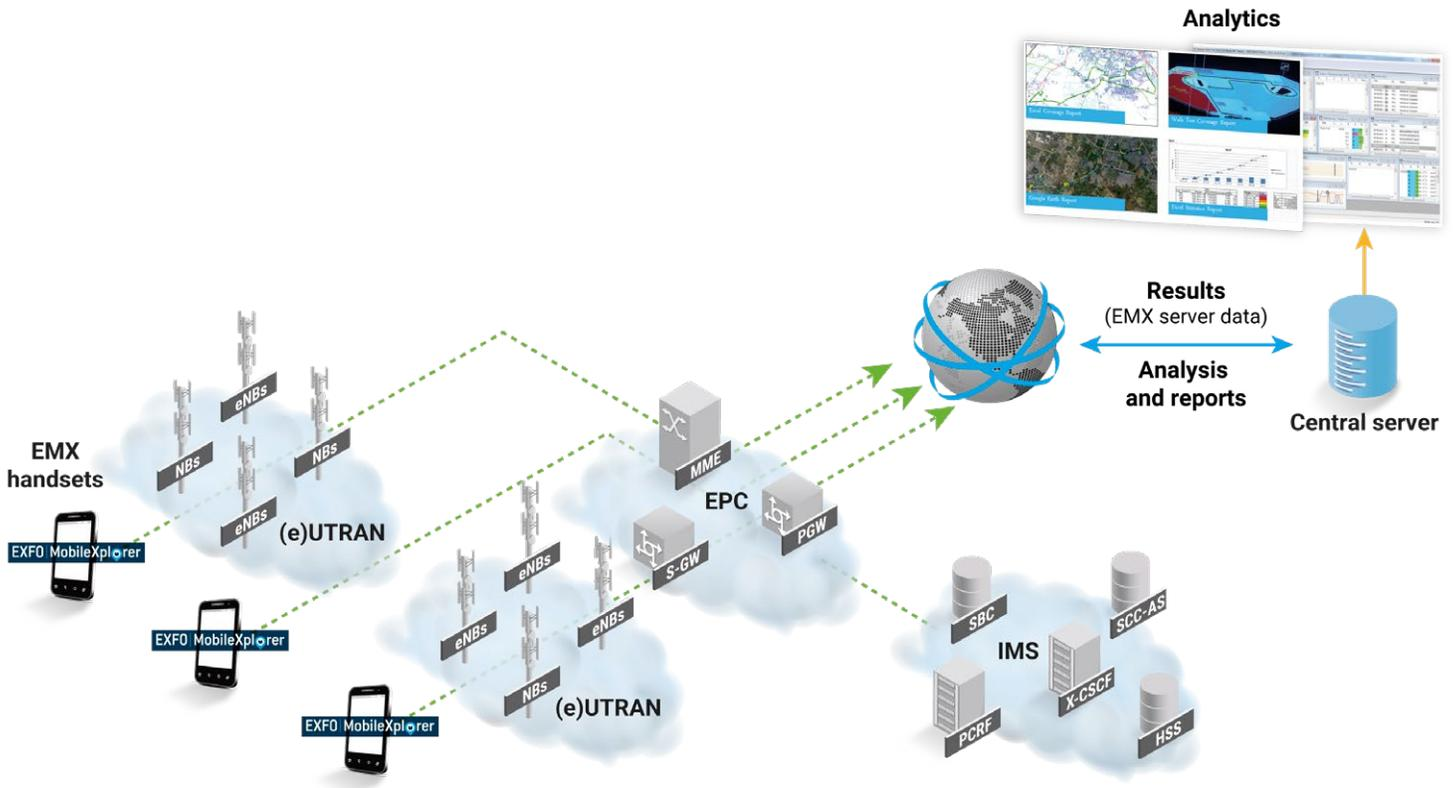
Figure 1. EXFO MobileXplorer network deployment
