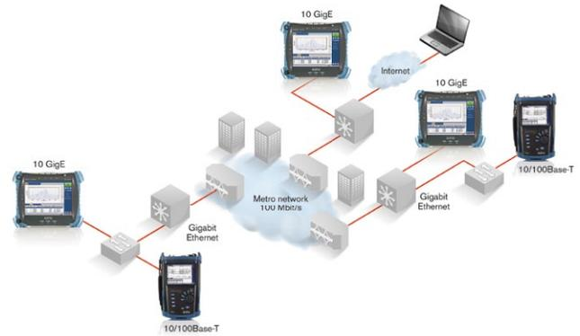
*Testing can be performed end-to-end or end-to-core, depending on the SLA. Remote testing is also possible.*
