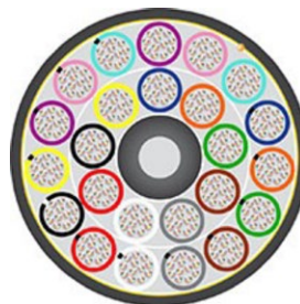
Example of a 3456 fibers cable.
