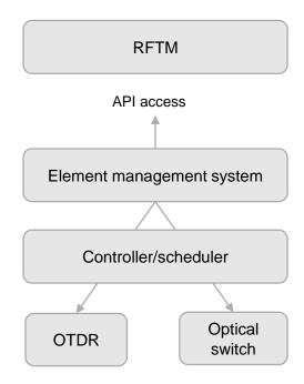
RFTM is based on micro-services and features well-documented APIs for integration with OSS/BSS applications as well as with other EXFO solutions such as SensAl.
