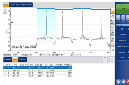
The FTB-5235 displays channel power, channel wavelength and OSNR. Above: example of CWDM network OSA display. Below: example of DWDM network OSA display.
