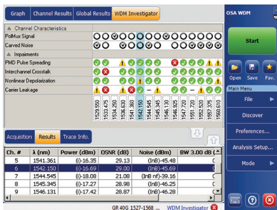
Figure 111. WDM Investigator reading showing a non-linear depolarization contributing to extended noise (OSNR e ).
