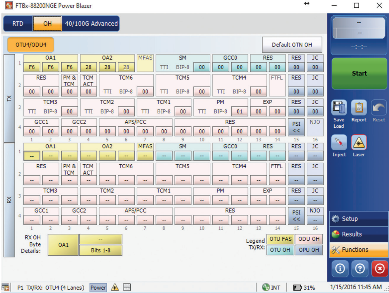
Figure 43. OTN overhead configuration.
