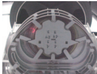
Figure 2-7. Macrobend detected with VFL
