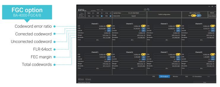
FEC encoded scramble idle metrics in the GUI
