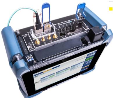
Most flexible and future-proof 1G to 800G dual-port test solution for lab and field applications, supporting current and next-gen pluggables.
