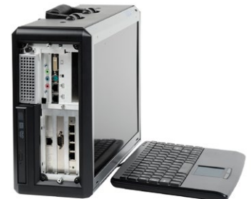
QA-T fitted with PCI-X NPU card
