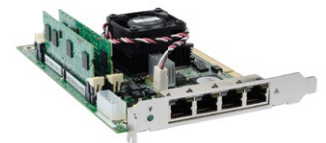
NPU-based interface card for connectivity with the SUT
