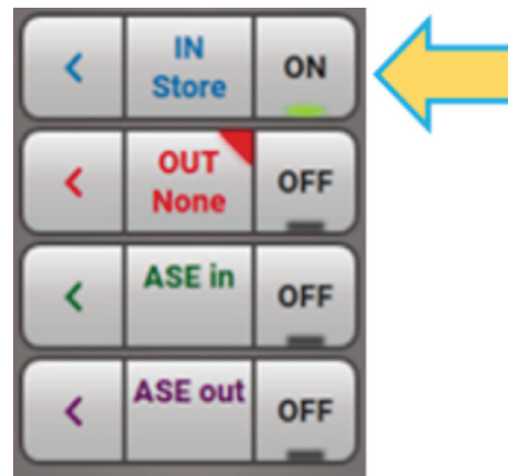
Figure 5. Storing the reference signal.
