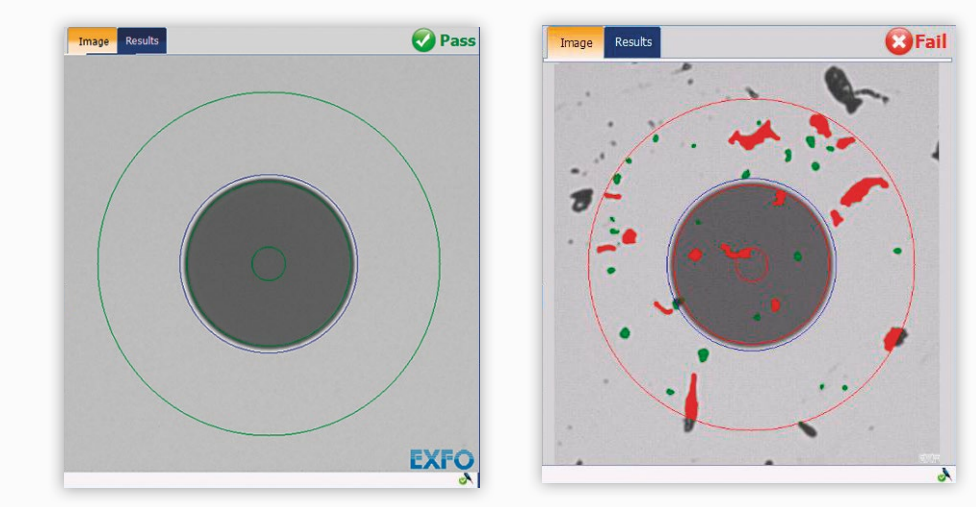
Figure 1. Functional, clean connector. Figure 2. Permanently damaged connector due to uncleanness.
