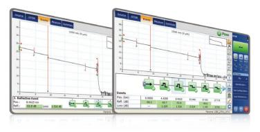
This improved version of linear view provides the flexibility to display both the OTDR graph and its linear view without having to toggle to analyze your fiber link.
