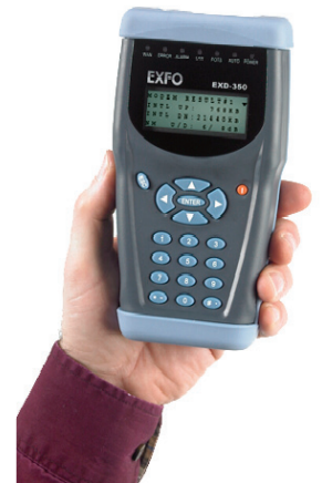
The EXD-350 Advanced ADSL2+ Tester
