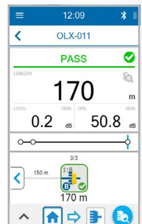
Testing from drop terminal towards splitter cabinet
