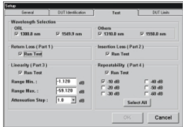
Typical tests performed on an attenuator
