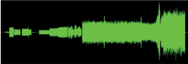
Figure 3. Spectrum of dial-up modem communication sequence
