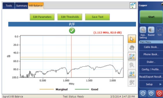
Figure 35. A measurement of the longitudinal balance on a local loop
