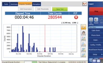
Figure 34. A measurement of counted impulsive noise hits vs. impulse duration.
